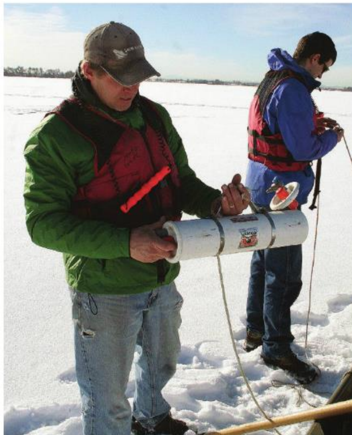
Steve Lundt demonstrates an apparatus used to take water samples to measure the quality of Barr Lake every half meter.
