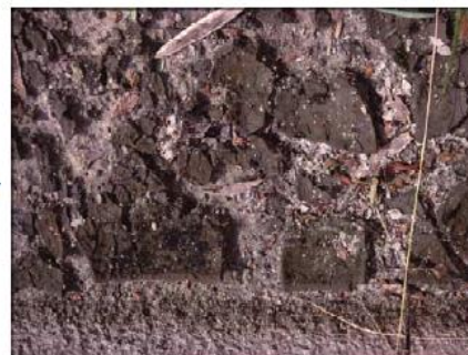
After 30 days Once completely dried, the floc forms into a rock hard material that will not re-dissolve
