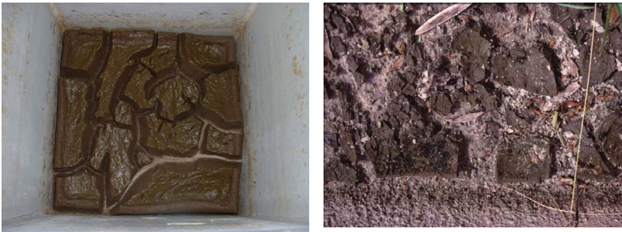
Figure 3. Alum Floc Drying Process.
